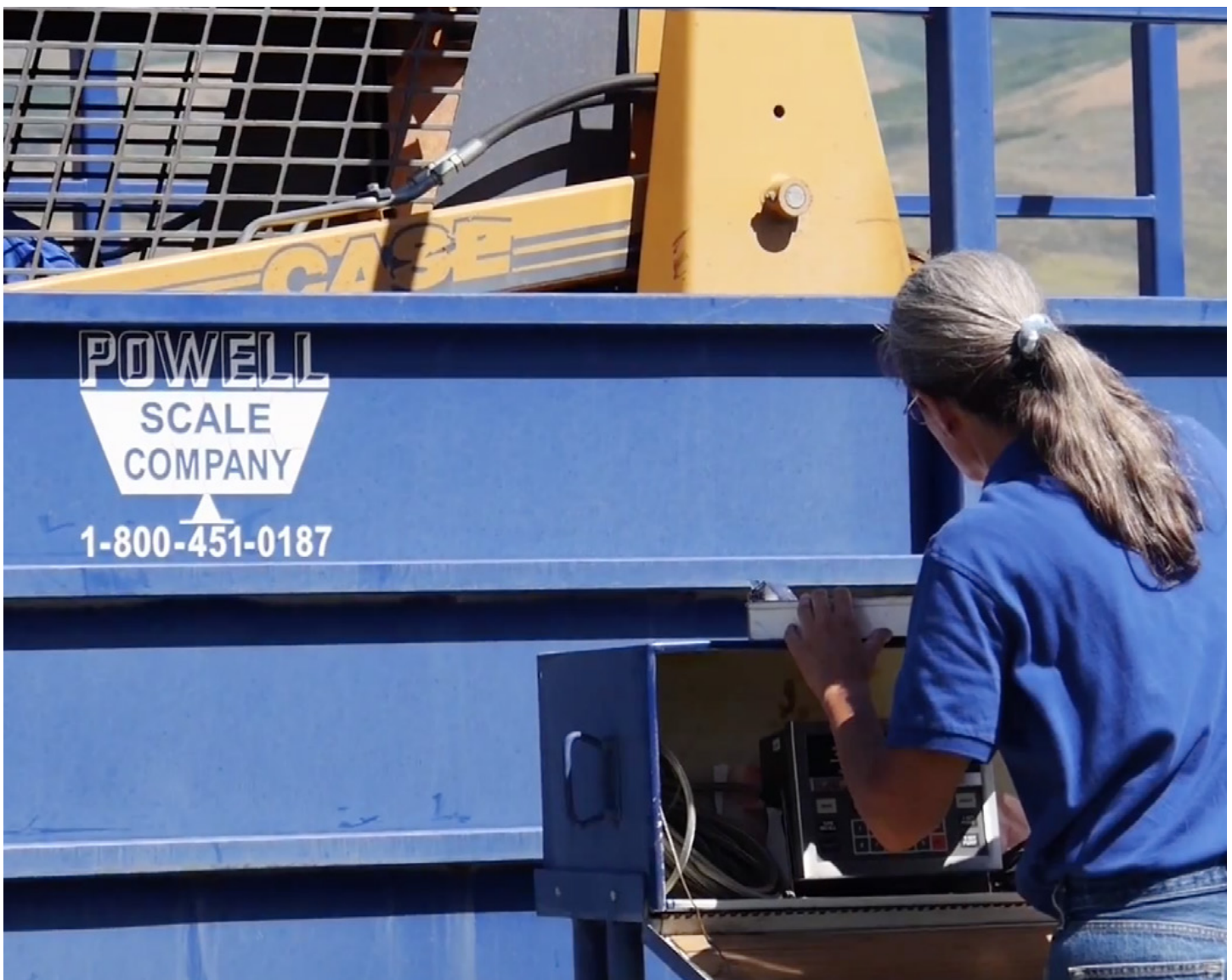
▲ Livestock scales are tested annually by NDA staff to ensure the scales accurately weigh cattle for market sales.
